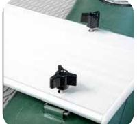
Place board over the bolts on one side of boat and work bolts through the holes.
