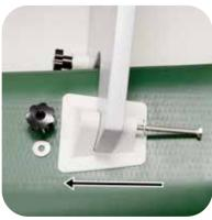
Push the 100mm (4") x M8 bolts with washer through the grommets and transom. If needed, push sides so transom holes align with arommet holes. A wrench is recommended for holding the bolt heads while tightening the threaded knob. When all four bolts are inserted, inflate the side chambers to the working
