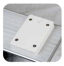
Attach Quick Release adapter block to aluminum board using M6 x 40 mm (1 ½") socket head screws, washers and locking nuts. The sides are tapered, install so that block and base can slide together.
