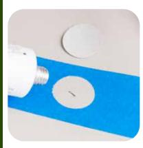
Apply glue to the patch and boat. Allow to dry 15 minutes. Glue must be dry to the touch. If glue layer is thin, apply second coat, allow to dry 15 minutes.
