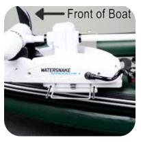
Place motor over Quick Release plate and insert locking bar. Locking bar must engage the clip. Follow manufacturer's instructions for deploying and stowing the motor. For Watersnake, see the next page of this manual.
